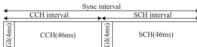
Fig. 2. Frequency channel layout of a 5.9 GHz WAVE system.
