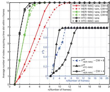
Fig. 4. The average number of nodes which acquire a time slot within  $n$  frames and  $F^{all}$  with  $CW = 4, 8,$  and  $10$  nodes.
