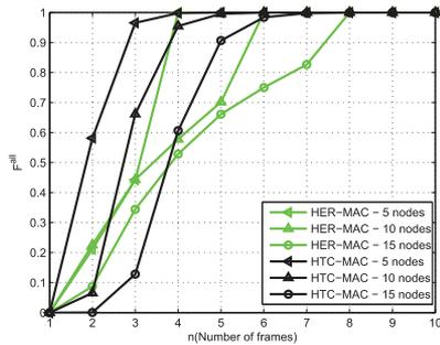
Fig. 5. Probability that all nodes acquire a time slot within  $n$  frames.
