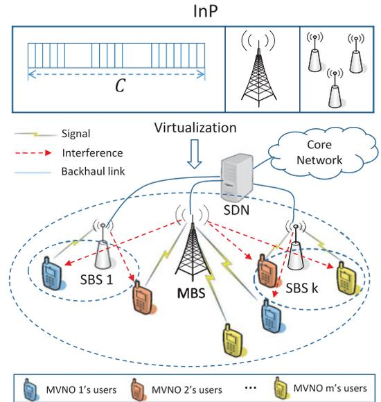
Fig. 1. System model: The InP owns the physical resource (i.e., spectrum and BSs), virtualizes these resources, and allocates to multiple MVNOs.
