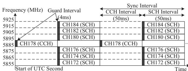
Fig. 1: Frequency channel layout of a WAVE system.
