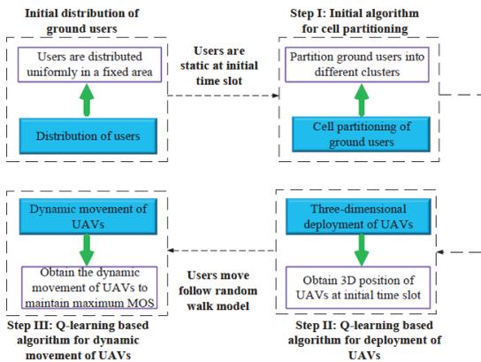
Figure 2. The procedure for solving the problem of deploying and movement design of multiple UAVs in [7]
