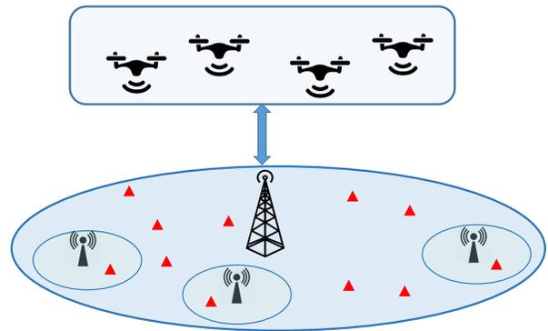
Fig. 1: System model of UAV-based heterogeneous network. The UAV pool is deployed over the terrestrial network consisting of MBS and TBSs. The small red triangles represent the mobile nodes uniformly deployed in the area.
