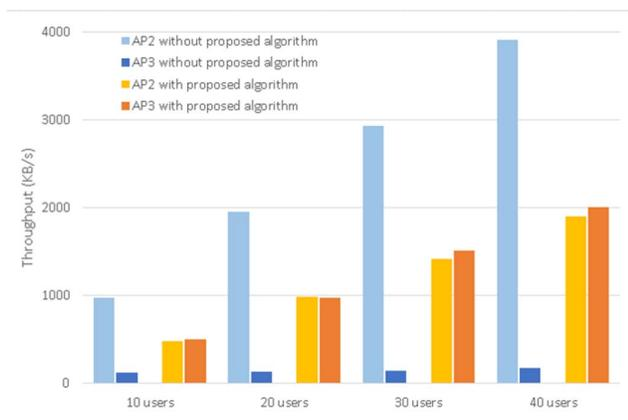
Fig. 7. Comparison of Backhaul link bandwidth of APs with existing algorithm and proposed algorithm
