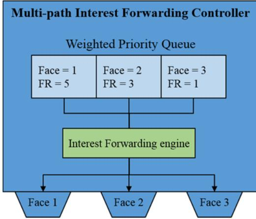
Fig. 2 Operation example of MIF controller
