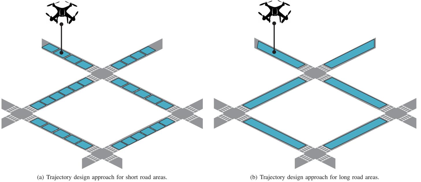
Fig. 2: (a) shows the trajectory design scheme where the whole are is divided into a set of location points and the UAV trajectory is developed by making decision at every location point to complete the trajectory. (b) shows a simplified trajectory design scheme where the trajectory design decisions are made only at the traffic intersections only to reduce the trajectory design computation complexity.
