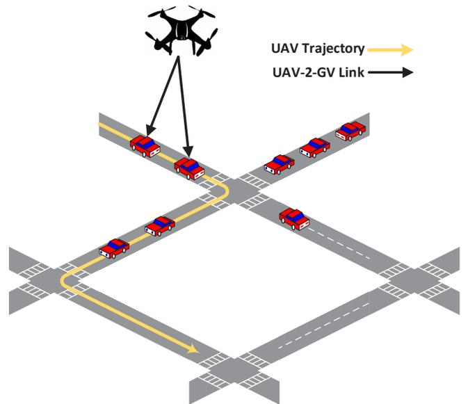
Fig. 1: System model representing the trajectory of the UAV to serve GVs. The suitable vehicles are associated with the UAV while the UAV is flying over the spots containing maximum number of vehicles.
