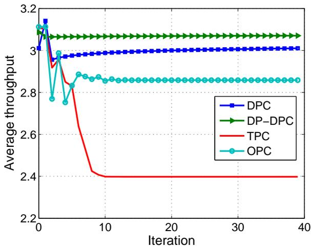
Figure 5: Comparison algorithms for target SINR of 10 dB
