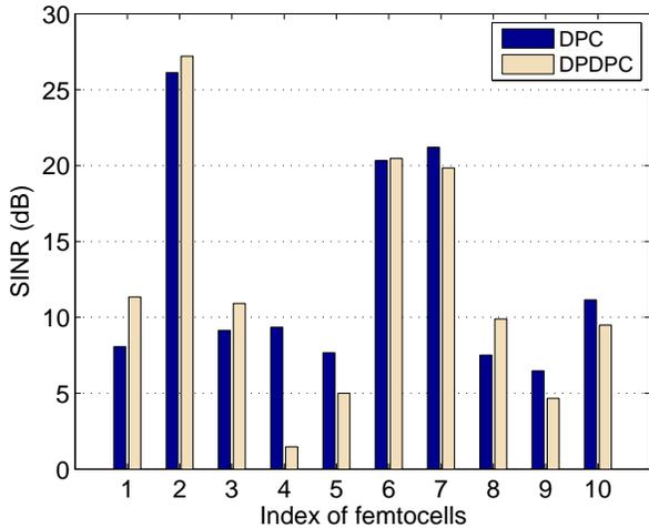
Figure 4: SINR for the DPC and DPDPDC algorithm for target SINR of 10 dB
