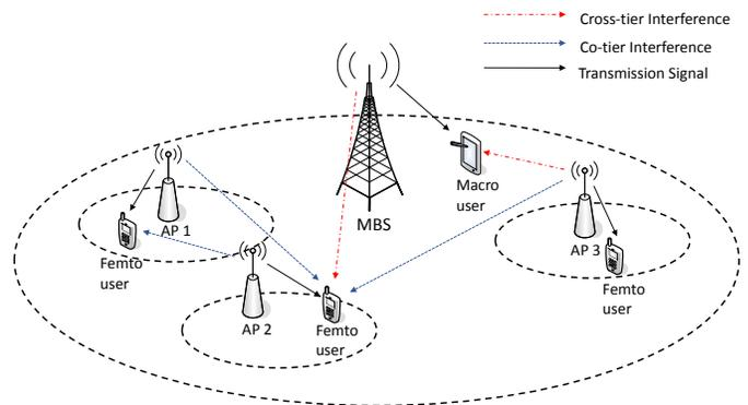
Figure 1: Network model with two-tier macrocell-femtocell
