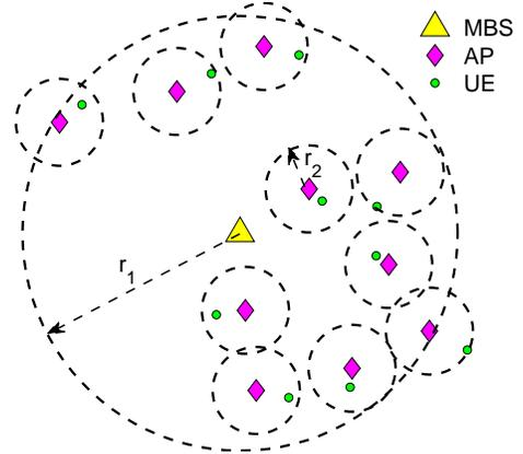
Figure 2: Network topology with two-tier macrocell-femtocell, where  $r_1$  and  $r_2$  are the radius of the macrocell and femtocells respectively.
