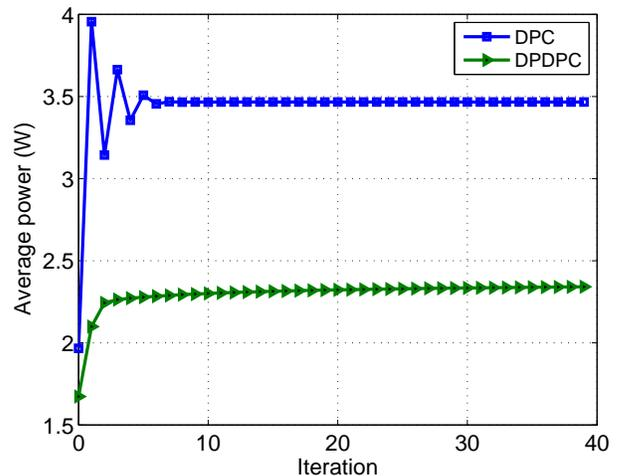
Figure 3: Average transmission power for the DPC and DPDPC algorithm for target SINR of 10 dB
