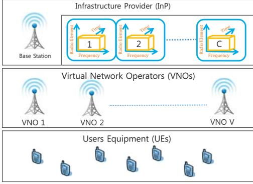
Figure 1: System model: The InP owns the physical infrastructure i.e., BS and subchannels which are virtualized and allocated to multiple VNOs.
