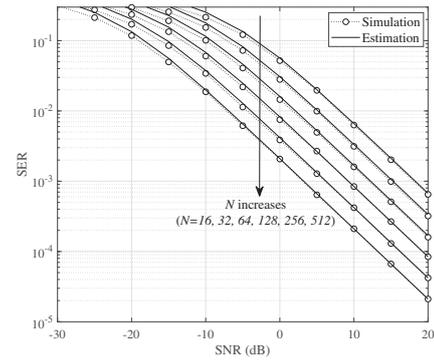
Fig. 4. Performance comparison of the average SERs resulting from the proposed modulation with different  $N$  values.
