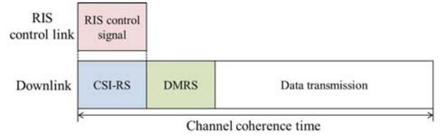
Fig. 2. Downlink frame structure at BS in considered RIS system.
