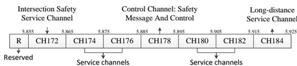
Fig. 1: DSRC spectrum allocation.
