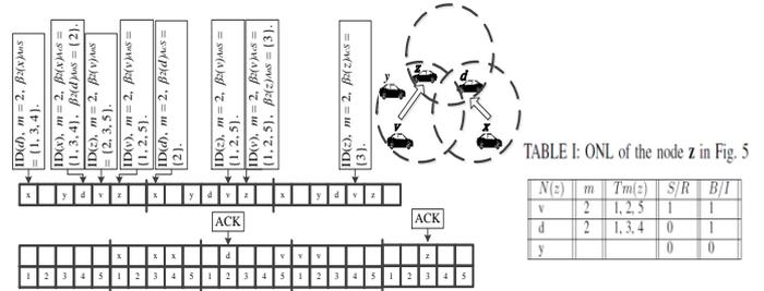
Fig. 5: A drawback of the VeMAC protocol on multi-parallel transmission.
