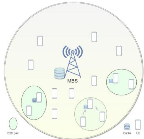
**Figure 1:** System diagram for outband D2D video offloading in cellular network.
