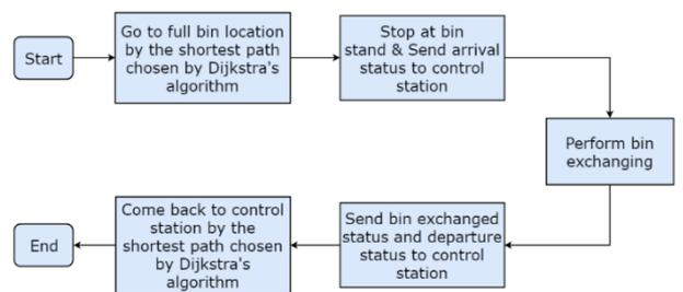
Figure 2. System Flow Diagram for Bin Exchanging Truck
