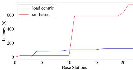
Figure 3. Latency comparison of Load Centric and SNR based approach
