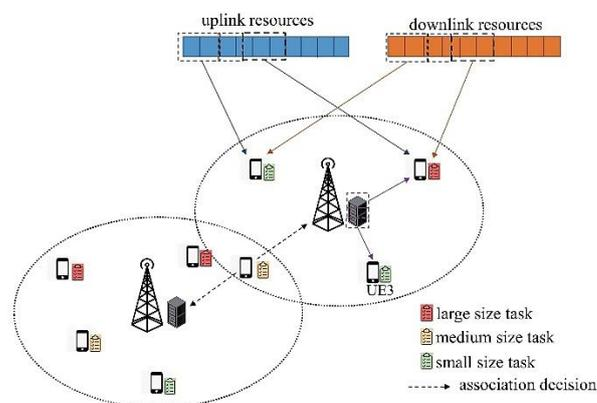
Figure 1. Task Association with Resource Allocation in MEC enabled Ultra-dense network
