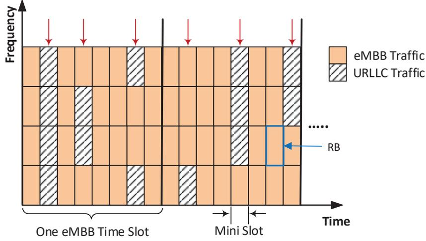
Figure 1: Puncturing approach for multiplexing of URLLC and eMBB
