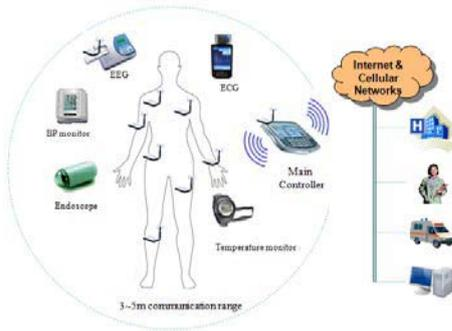
Fig 1. Structure of a BAN.
