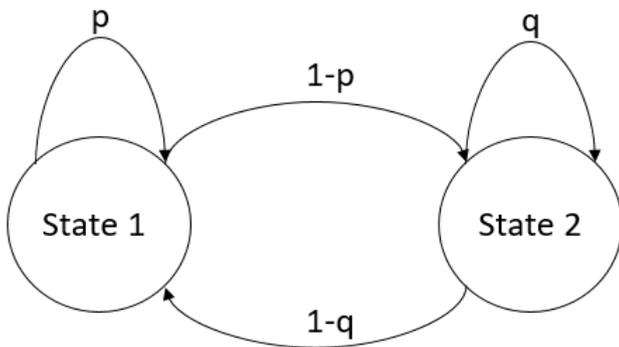
Fig 2: State Transition Diagram
