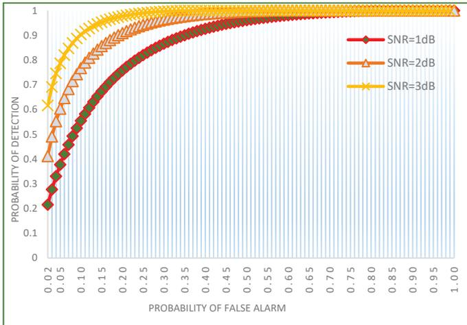
Fig. 1. Probability of PU detection vs. probability of false alarm with different SNR values.
