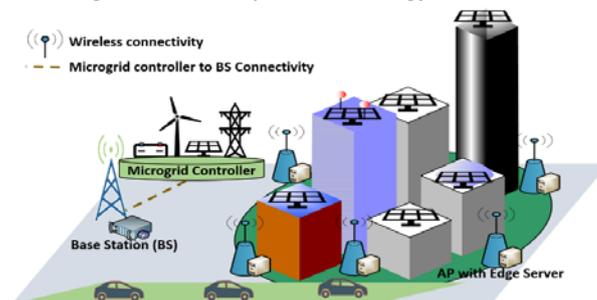
Figure 1: MEC-enabled microgrid-powered smart city scenario
