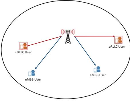
Fig. 1. System model of URLLC and EMBB coexistence network.
