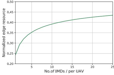
Fig. 2: Impact of the increase in the number of IMDs per UAV on normalized edge resource trading point.
