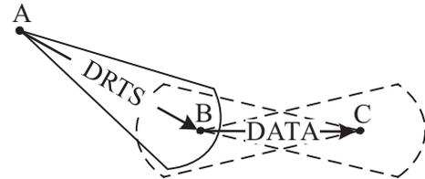
Fig. 5: Deafness due to directional antennas.
