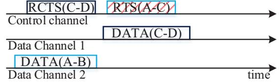
Fig. 4: Missing receiver due to multi-channel environment.
