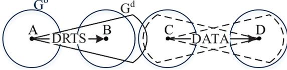
Fig. 1: Hidden terminal due to the asymmetric antenna gains.
