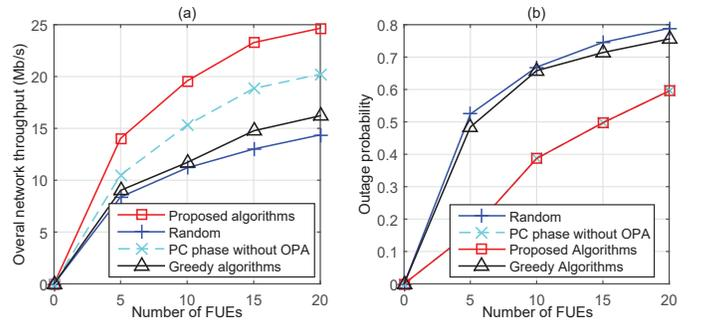
Figure 4: Total throughput and outage probability in uplink CFN versus number of FUEs  $N$  when  $M = 5$ ,  $K = 5$ ,  $I_k^{k,th} = -70$  dBm.
