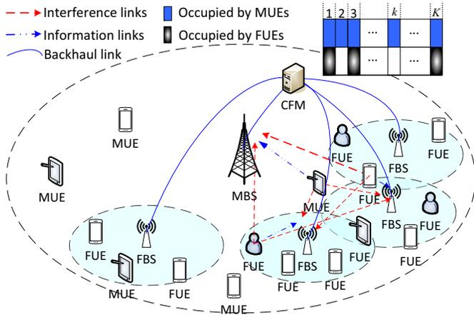
Figure 1: System architecture of a cognitive femtocell system.
