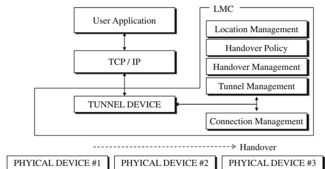
**Fig. 1** Functional architecture of LMC
